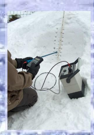
The sensor is a steel fork used as a microwave resonator. Snow Fork measures the electrical parameters: resonant frequency, attenuation and 3-dB bandwidth.
